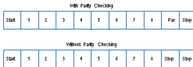
Figure 6 Bit Order (RTU)
